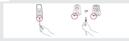
Assemble the remote control cradle onto the frame and place the remote control onto the cradle. Check the connectors for the SD card, remote control and the external projector and connect appropriately.
